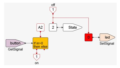
Initially this super block is activated through its activation input port. This process changes the state number to 2 and sets to zero the LED signal. Subsequent activations come through the activation signal A2. No output activation is generated until the button signal goes positive. The output activation signals **on**, then enters the **LED-on** super block.
