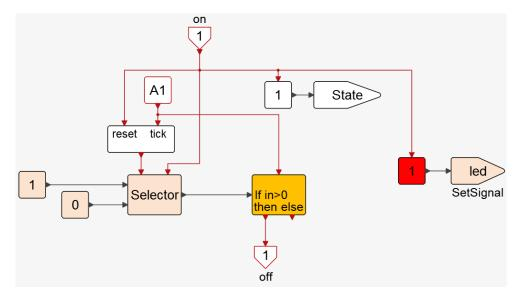
The on signal changes the value of state to 1 (thus deactivating the state represented by the LEDoff super block and activating the LED\_on super block state. It also sets the signal LED to 1 (turning on the LED) and resets a counter.
